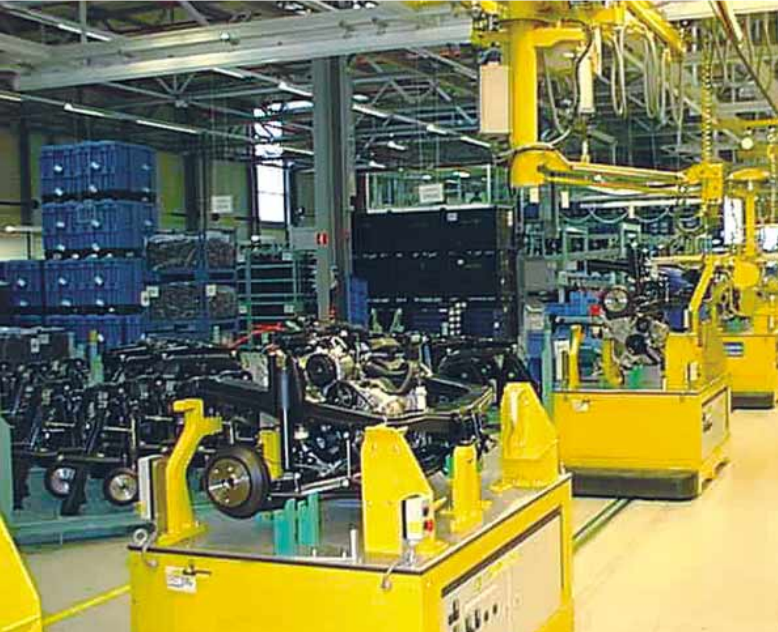
Assembly of the rear axle drive module for the smart® in Hambach, France (Fig. 1)
