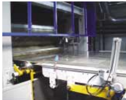
Finished base plate exiting a hot pressing line (Fig. 5)
