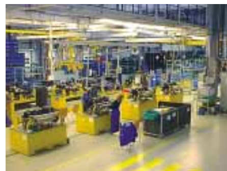
smart ® assembly line with oil filling and final inspection (Fig. 5)
