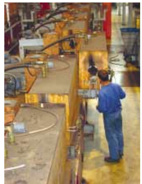
Easy-to-maintain induction heater (Fig. 3)
