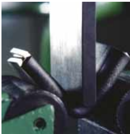
Bending test to determine extreme load capacities during cold forming (Fig. 2)
