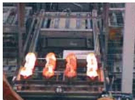
Tray with hot crankshafts on the way to the cooling shelves (Fig. 6a)
