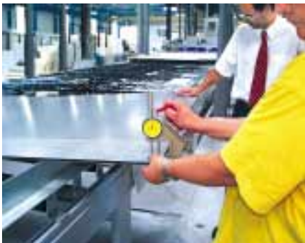
Checking the polypropylene base plate (Fig. 4)
