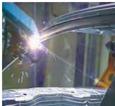
Laser welding process (Fig. 2)
