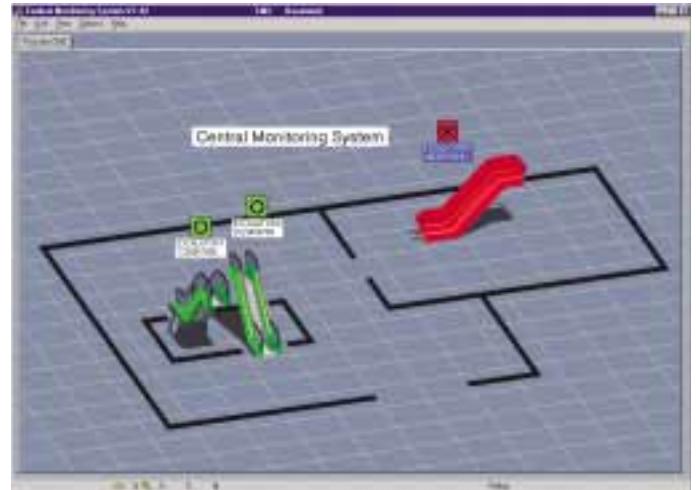
Failure information via CMS (Fig. 6)
